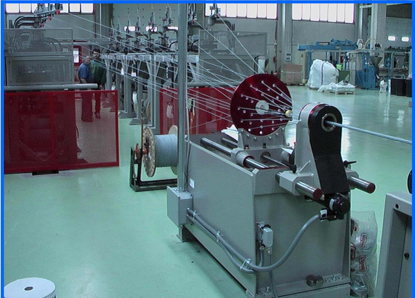
LIGNE D'ASSEMBLAGE A SIMPLE TORSION POUR CABLES SPECIAUX, MICRO-COAXIAUX, MULTI L.A.N. ET CABLES A FIBRES OPTIQUES. LA LIGNE EST ALIMENTEE' AVEC DEROULEURS A DETORSION COMPLET 100% OU ,A VOTRE CHOIX, LA DETORSION PEUT ETRE PROGRAMME' AVEC POURCENTAGES PLUS BAS. LA LIGNE EST LOGIQUEMENT PREDISPOSE POUR L'APPLICATION DE PLUS RUBANS LONGITUDINAUX EN PLUS D' AVOIR LA POSSIBILITE' DE RUBANER A HELICE FERMEE' OU CONTROVERSEE'.
